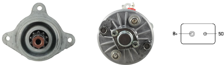
PRESTOLITE Type 24V 7,80kW 10T CW
